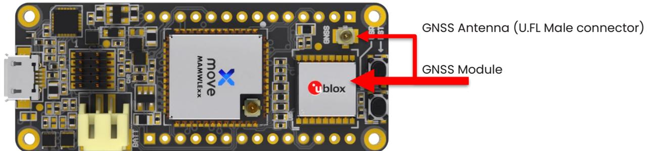
The *MAX-M10S* module integrates an LNA + SAW filter and so it is suitable for passive antennas, and thanks to its low power consumption is a perfect fit for battery-powered applications.
