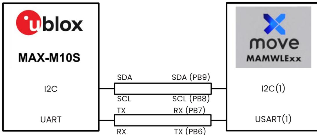
This GNSS module offers others GPIO pins that you can use: TIMEPULSE, EXTINT, RESET\_N. They are connected as follow:
